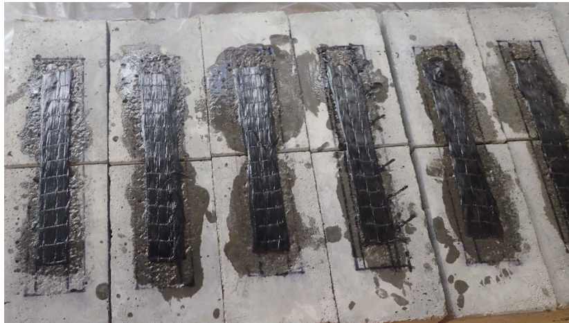
Figure 3.8: Insertion of CFRP on the tension surface of the beam specimens by wet layup process
