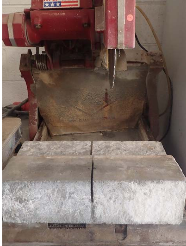
Figure 3.6: Insertion of notch in the midspan of the small beam specimen
