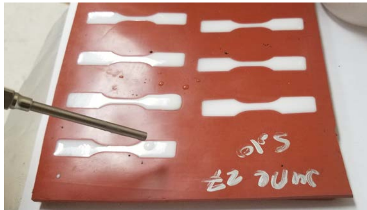
Figure 3.2: Epoxy injected into rubber mold
